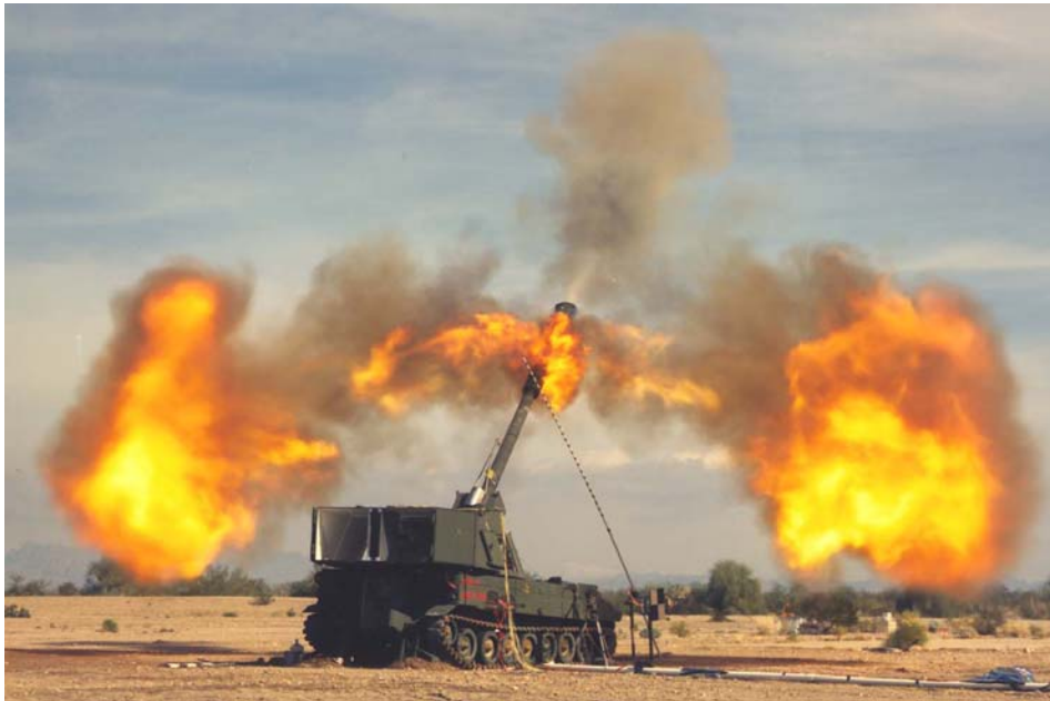
Figure 17: Gas flow deflection by a high efficiency muzzle brake
